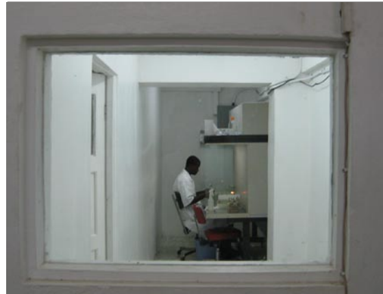
Cultures are taken in a laminar flow hood in effort to maintain a sterile environment
